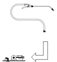
2. Attach the inlet tube to the fitting located on the bottom of the sprayer base plate.
