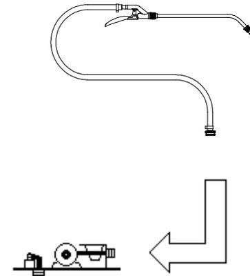
2. Attach the inlet tube to the fitting located on the bottom of the sprayer base plate.
